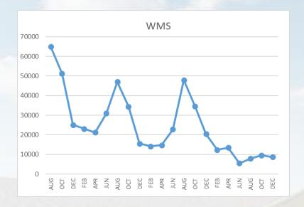
The WMS chart includes the following 7 meters: 755 Park high and low flow, BO and TEAM High, PIT house, bus barn, athletic field, and DO. All of these meters are totaled on the WMS graph, but each data point is recorded separately to aid in identifying leaks.
